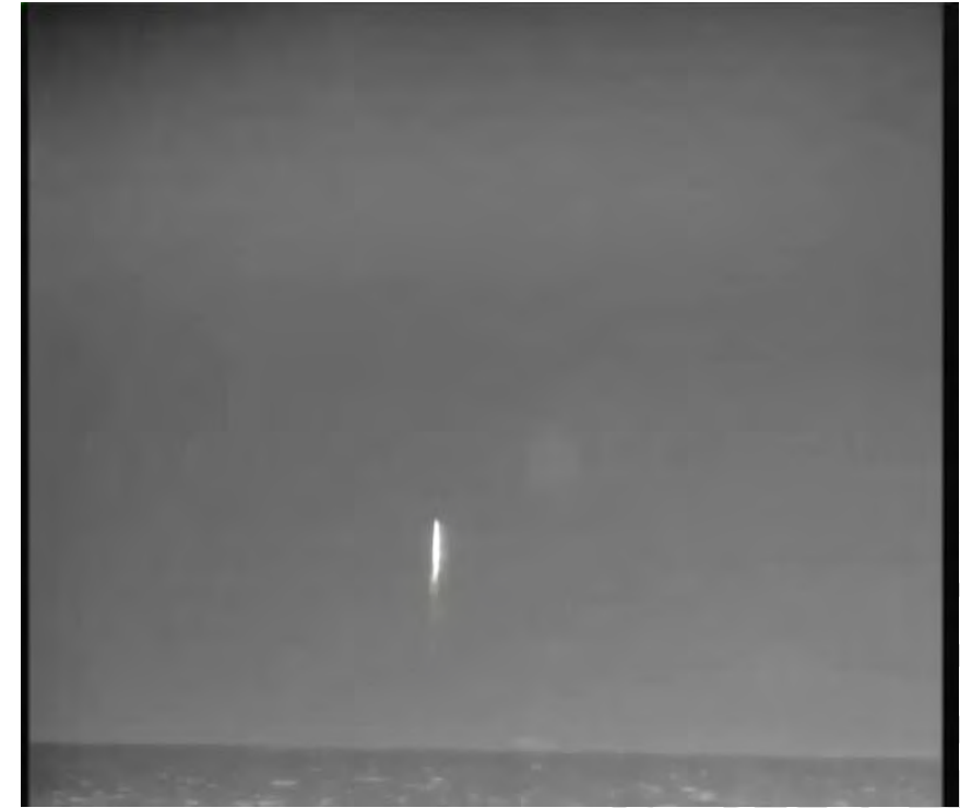
SpaceX rocket captured w 75mm lens on BAE 12um 640x512 camera- 12 mile distance
